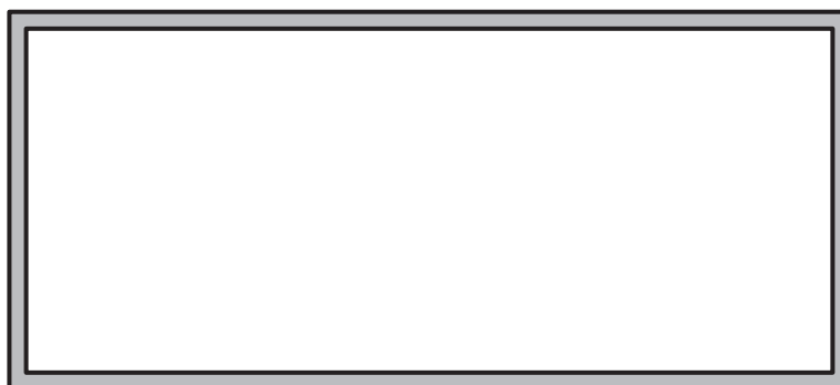
TUBO RECTANGULAR 100 x 45 x 2 mm.
